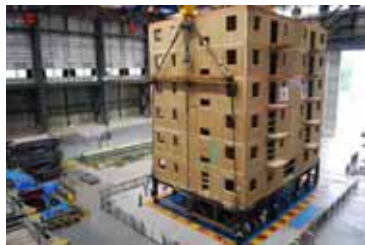
Full-size condominium building positioned on the shake table and ready for testing. Photo by John van de Lindt, Colorado State University.
